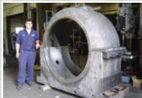
Large rebuilt ball mill trunnion housing
