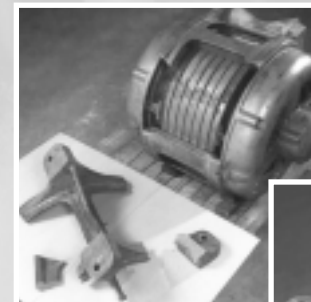
Broken 600 hp electrical motor housing
