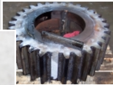
Broken tooth on a pinion gear
