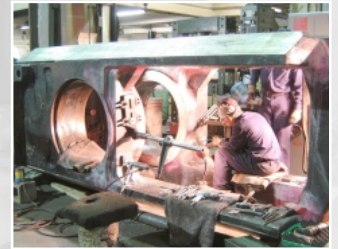
35,000 lb forging press ram being repaired, cast iron or cast steel - no problem
