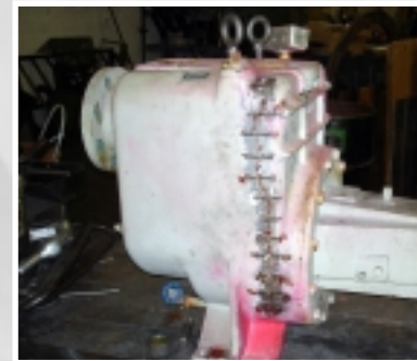
Damaged pump in the process of being repaired; locks and lacing being inserted
