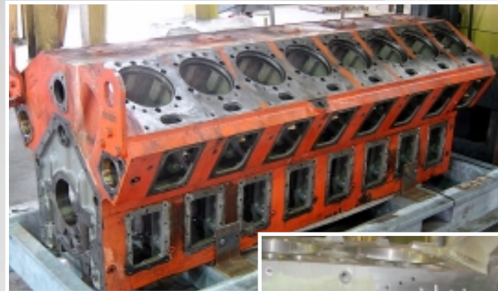
16 cylinder diesel generator to be repaired
