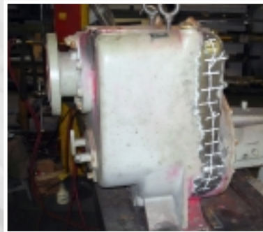
Repaired pump that has passed pressure testing, with repair highlighted for clarity
