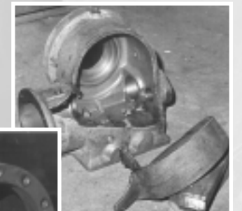
Broken valve body
