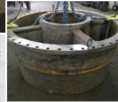
Hub repaired by metal locking process
