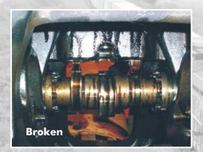
Crosshead Guide damage can occur for various reasons. Some of the more common reasons are: liner failure, improper lifter lubrication or catastrophic failure of a neighboring component such as a broken connecting rod or cam section.
