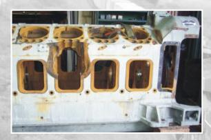
Crankcase Window damage occurs when a connecting rod fails and becomes wedged between the window and the crankshaft. The window is typically blown outward resulting in local crosshead guide damage. This is our most demanding repair as alignment of the replacement piece is critical for correct operation.
