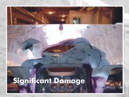
Pan Rail and Interior Wall & Rib repairs are usually caused by a broken connecting rod and/or cam section.
