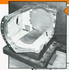
Accidental wedging of the crosshead, forced the top of the crosshead extension out Since the crosshead quide is an integral part of the main frame, the options or repair are few. Reattachment, particularly by use of heat (such as welding), would not only be inadequate for the strength required, but would present problems of alignment through distortion. which usually follows welding or brazing procedures.
