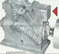
The completed elevator gear box housing, repaired and as strong as new. Photo shows area of repair "touched-up" to emphasize photography. Repair area is actually difficult to detect.
