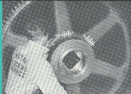
Typical repair on 60" Bull Gear, broken through spokes where fracture often occurs.
