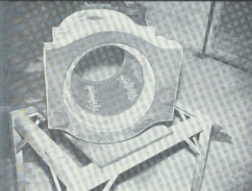
Bearing Housing from main roll of rubber pulverizer. Sealed against water pressure.
